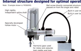
A totally beltless structure was achieved by using a ZR axis direct coupling structure. This direct drive structure drastically reduces wasted motion. It also maintains high accuracy over a long period of time. It ensures maintenance-free usage for extended periods with no worries about belt breakage, stretching or deterioration with age (feature applies to all XG series models and the YK180X/YK220X).
