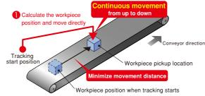
Operating conditions: YK500XG / Payload mass 1 kg (total of tool and workpiece) / Horizonta ment 250 mm / Vertical movement 1 mm / Conveyer speed 100 mm/sec
